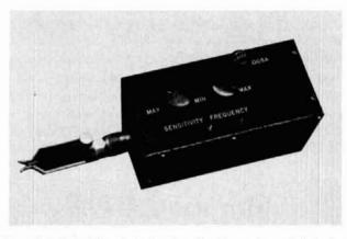
Complete fluted line detector showing the probe and detector.
